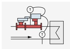
Control Signal DDC controls the thermal power setpoint as long as the delta T is above the delta T setpoint
