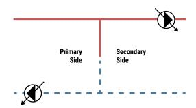
Figure 53: A simple depiction of a primary secondary ciruit with an hydaulic separator.
