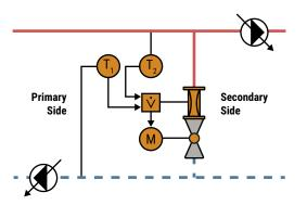
Figure 54: Shows an energy valve monitoring the temperature spread of the primary and flow through the separator.
