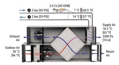
Figure 63: AHU at design operation
