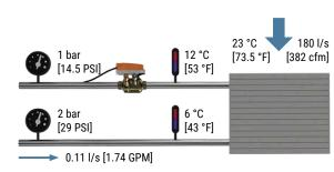
Figure 86: FCU at design operation
