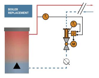
Figure 131: Condensing Boiler equipped with air bubble tight EV.
