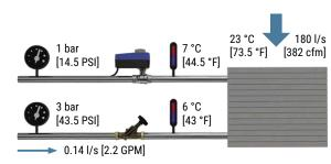
Figure 85: FCU with valve overflowing
