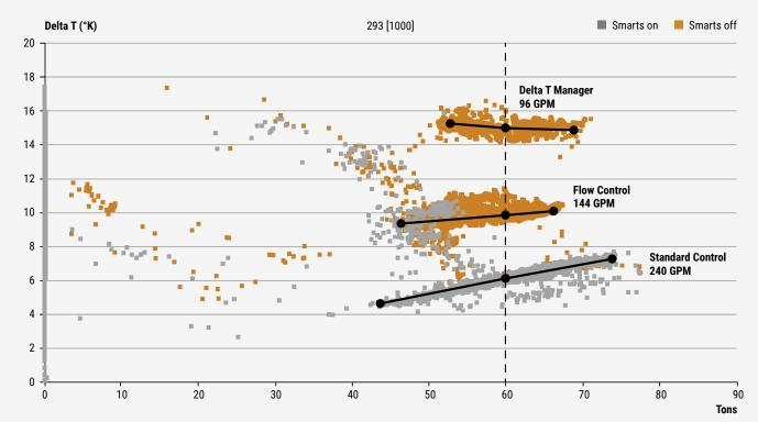
Figure 34: Operating conditions (delta T, load) of the valve in different control modes.
