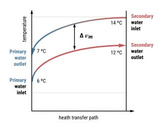
**Figure 75:**  $\Delta \vartheta_m$  average temperature difference design flow
