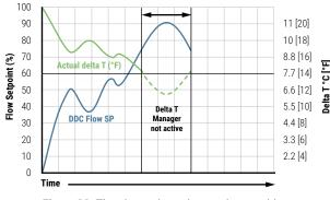
Figure 32: The above chart shows what would happen if the Delta T Manager was not active. Here the DDC setpoint drives the demand so high that the delta T will drop below the desired setpoint of  $14\,^{\circ}\text{F}$
