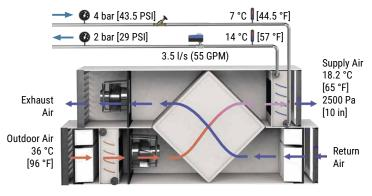
Figure 62: AHU with valve overflowing
