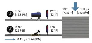
Figure 84: FCU at design operation
