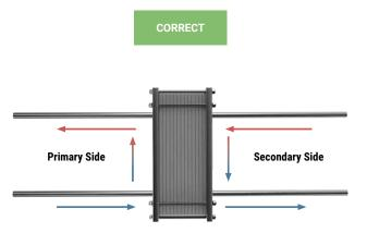
Figure 72: Cooling transfer station contraflow
