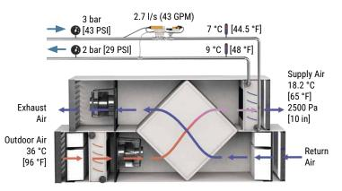
Figure 64: AHU without valve overflow
