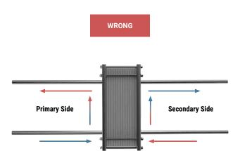
Figure 70: Cooling transfer station direct flow
