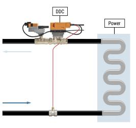
**Figure 28:** Power Control of the Energy input to a Consumer
