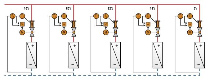
Figure 52: Shows the thermal index, the most open valve, which selected by the BMS.
