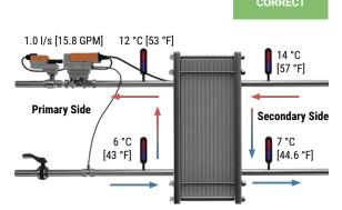
Figure 79: Dynamic balancing with Delta T Monitoring
