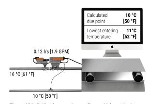
**Figure 101:** Chilled beam using an Energy Valve, with the BMS calculating the dewpoint with the input from a room-sensor
