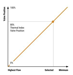
Figure 51: Shows a simple method of selecting flow temperature based on thermal index valve position.
