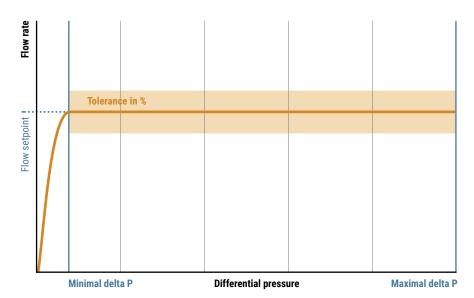
Figure 83: Dynamic Balancing of a FCU
