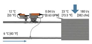
Figure 88: FCU with delta T optimized valve flow
