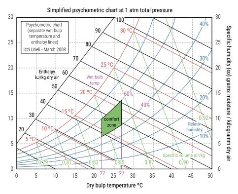
Figure 97: The dewpoint is depending on the air temperature and humidity
