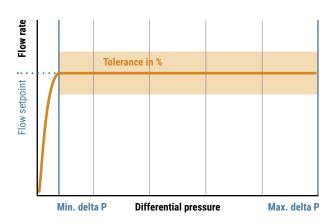
Figure 58: Dynamic Balancing assures an accurate flow rate
