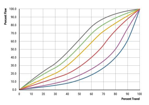
**Figure 25:** The distortion of the characteristic that could occur if the valve is left in position control.
