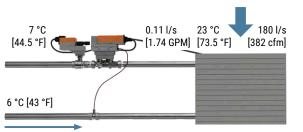
Figure 87: FCU without water overflow
