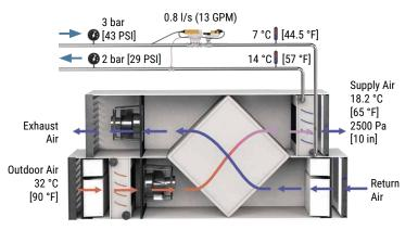
Figure 65: AHU with delta T optimized valve flow
