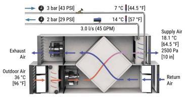
Figure 61: AHU at design operation
