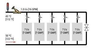
Figure 112: Mechanical balancing valves only allow for a static balancing of the total flow to the floor, flow rates to individual units is unknown.
