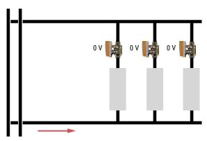
**Figure 119:** PIQCV valves instead of control valve and balancing valve combo
