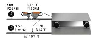
Figure 100: Chilled beam using an Energy Valve
