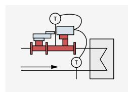
Control Signal DDC controls the flow as long as the delta T is above the Delta T Setpoint.
