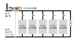
Figure 113: With an EV the branch flowcan be measured when each valve is opened, allowing verification.
