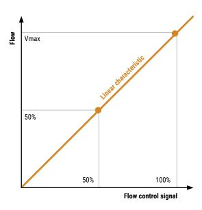
**Figure 26:** Flow Characteristics related to Flow Control Signal
