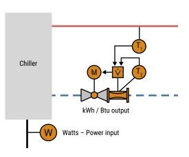
Figure 134: Chiller / Heat Pump with indicated cooling circuit
