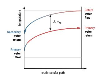
**Figure 73:** Δϑ<sub>m</sub> average temperature difference contraflow
