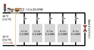
Figure 115: With an EV both leaking short-stroke valves or an open bypass can be clearly identified
