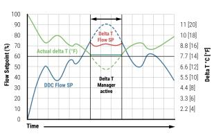
**Figure 35:** "Scaling Delta T Manager" scales the delta T set point depending on the current flow rate.
