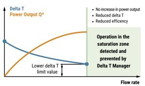
**Figure 60:** Improved energy-efficiency with the Energy Valves™ Delta T Manager enabled.
