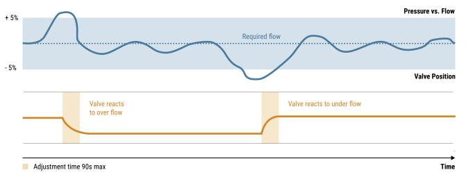
Figure 20: Reaction of ePIV to pressure changes
