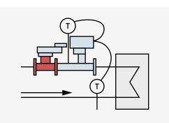
Control Signal DDC controls the valve position as long as the delta T is above the Delta T Setpoint
