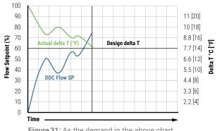
**Figure 31:** As the demand in the above chart starts to rise and the flow changes, the actual delta T starts to decrease
