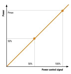
**Figure 29:** Control characteristics in Power Control Mode
