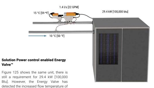
Figure 125: CRAC unit with higher supply temperature (for energy savings)
