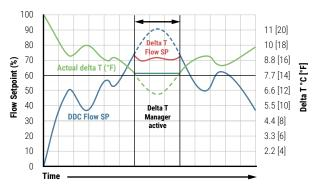
**Figure 33:** Delta T Manager detects low delta T, goes active, managing the flow to maintain the minimum delta T
