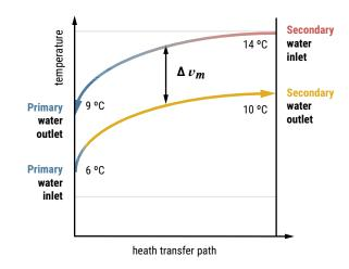
**Figure 77:**  $\Delta \vartheta_{m}$  average temperature difference overflow
