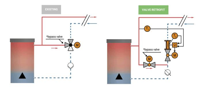
Figure 129: Boiler with a globe valve \*bypass valve to prevent condensation during start up
