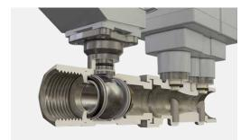
**Figure 14:** Electronic PI valves have a simple flow path, removing flow direction changes significantly improves dirt tolerance.
