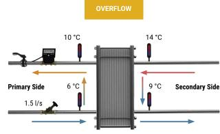
Figure 76: Overflow caused by pressure fluctations
