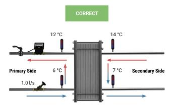
Figure 74: Typical design flow (cooling application)
