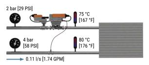
**Figure 108:** FCU in cooling mode using a pressure-independent EV
