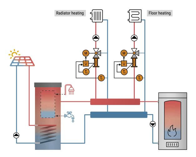
Figure 128: Typical hydronic schematic of a Central Heating Plant combining multiple alternative and renewable energy sources
